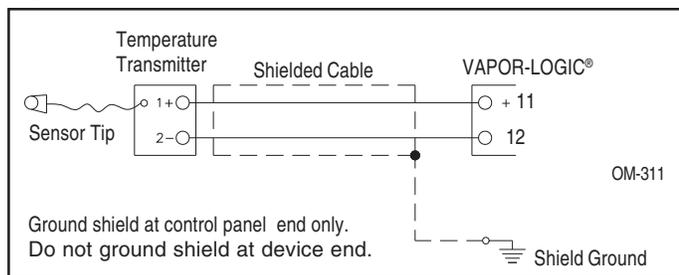
**OPTION: Cold Snap RH Offset** (Shielded cable recommended, see note). When selected as an option, DRI-STEEM provides a cold snap temperature transmitter. The letter "T" in your nomenclature code activates this option: ILIIOA7OTOX.
