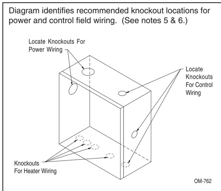
**CAUTION** - When providing holes and knockouts in the control cabinet, protect all internal components from debris and vacuum out cabinet when finished. Failure to comply with this warning may damage sensitive electronic components and void the DRI-STEEM warranty.
