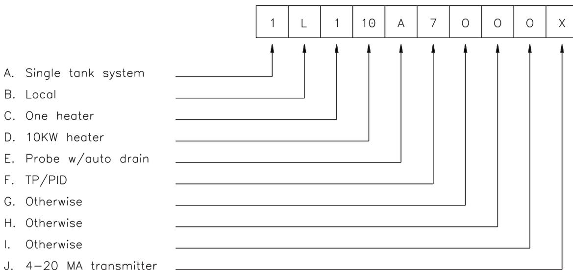
Code number for typical VAPOR-LOGIC slave control board 1N110A7000N
