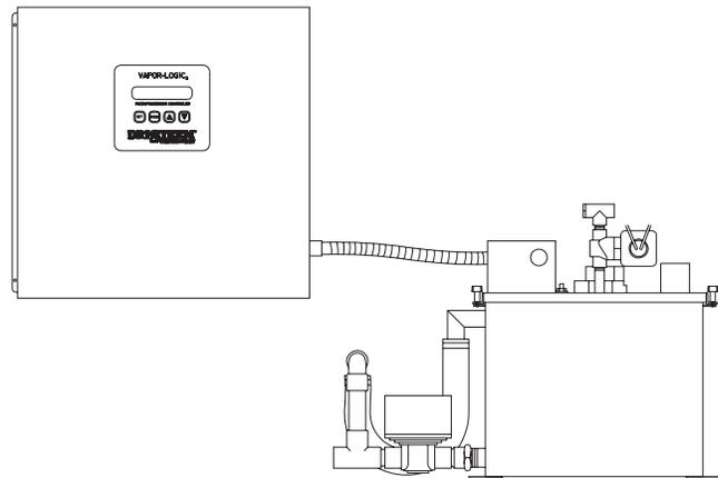
**Figure 4-3:** The VAPOR-LOGIC<sub>2</sub> key pad is mounted on the front of the VAPORMIST cabinet for easy access.
