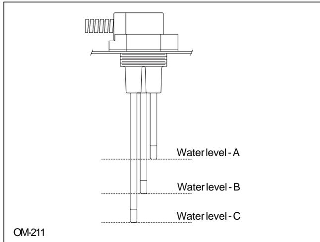
A conductivity probe system allows VAPOR-LOGIC<sub>2</sub> to control water levels for optimum operating efficiency. The three-probe system is monitored by the VAPOR-LOGIC<sub>2</sub> control, which performs all the necessary logic and timing functions to provide total water level control and safety shutdown.
