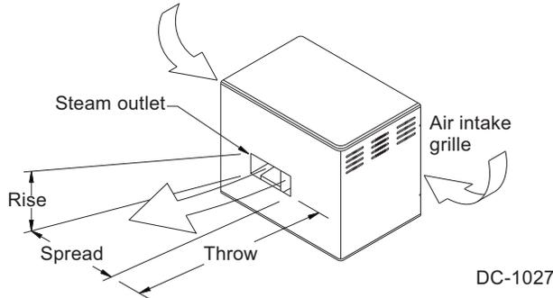
As steam is discharged from the SDU-E, it quickly cools and turns to a visible fog that is lighter than air. As this fog is carried away from the SDU-E by the airstream, it tends to rise toward the ceiling. If this fog contacts solid surfaces (columns, beams, ceiling, pipes, etc.) before it disappears, it could collect and drip as water. The greater the space relative humidity, the more the fog will rise, throw and spread.
