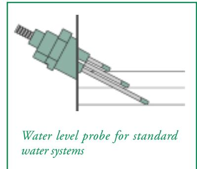
levels. For the probe to sense water levels, the water in the tank must have a conductivity of at least 100  $\mu\text{S}/\text{cm}$  (water with hardness of at least 2 grains/gallon).
