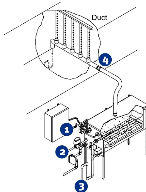
1. Tap, softened, or DI/RO water fills the evaporating chamber through the fill valve. This is the water that will be converted into steam for humidification.
