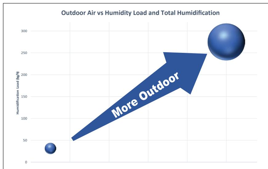
2. More water and energy are needed to humidify when the percentage of outdoor air is increased
